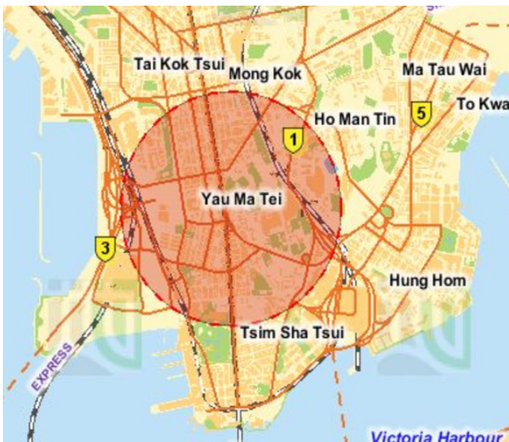
Figure 4. A circle with radius of 1km (to protect adjacent band operation of small-cell indoor terminals)
