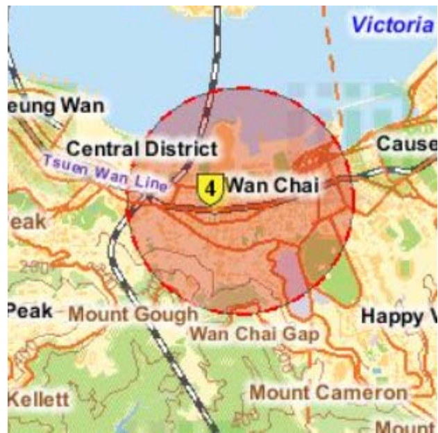
Figure 5. A circle with radius of 1km (to protect adjacent band operation of small-cell indoor terminals)
