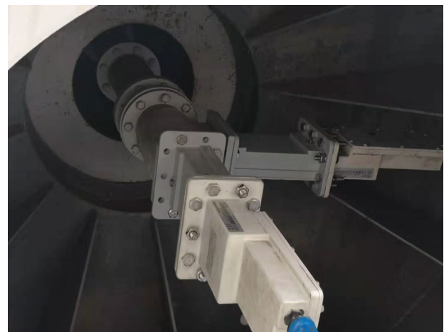
Figure 10. AsiaSat BPFs installed on two different antenna feeds. Both the V and H-polarization paths are installed with AsiaSat BPFs
